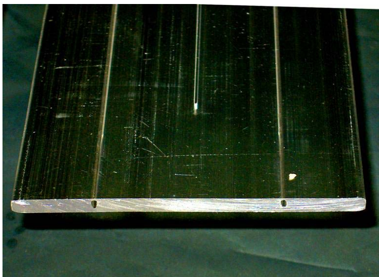
Figure 4: A pair of extruded scintillator strips for the TCMT.
