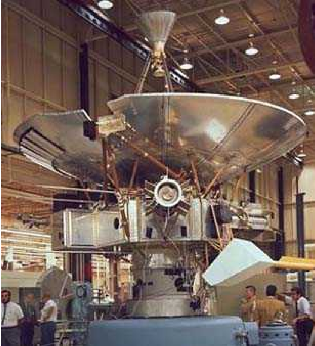
The Pioneer F spacecraft during a checkout with the launch vehicle third stage at Cape Kennedy. Pioneer F became Pioneer 10.
