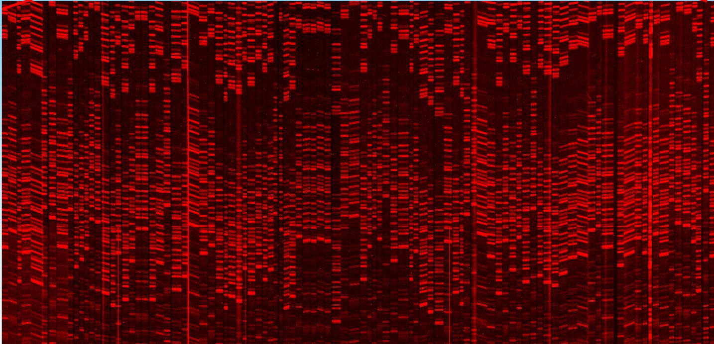
Using custom-milled slitmasks with **DEIMOS** we are obtaining spectra of  $\sim 130$  targets at a time. A total of 400 slitmasks was required for the survey; we can tilt slits up to 30 degrees to obtain rotation curves.
