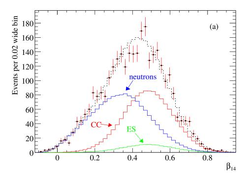
Figure 7: Event isotropy variable,  $\beta_{14}$ , distribution for neutrons (from NC reactions and background), and CC and ES reactions. Large values of  $\beta_{14}$  indicate less isotropic light distribution in an event. The data points show the neutrino data from the salt phase. The dashed histogram is the sum of the Monte Carlo probability density functions scaled by the fitted numbers of events.
