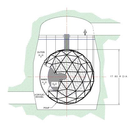
Figure 1: Schematic drawing of the SNO detector. The detector is described in the text.
