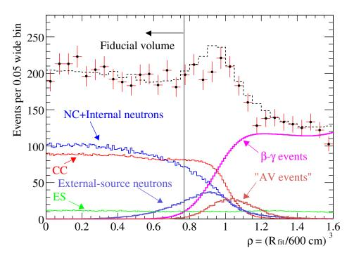
Figure 12: Distributions of volume-weighted radius,  $\rho$ , for neutrons, CC events, and ES events, summed MC PDFs (dashed histogram) and real neutrino data (data points). The  $\beta - \gamma$  and "AV" events are sources of background whose magnitudes are determined separately from this fit. The acrylic sphere is at  $\rho = 1$ .
