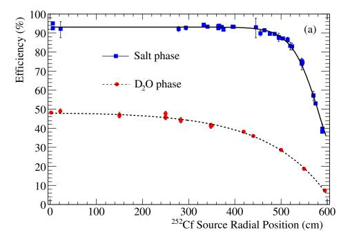
Figure 6: SNO's neutron capture efficiencies for the pure  $D_2O$  and salt phases. The neutron capture efficiency is measured with neutrons from a radioactive <sup>252</sup>Cf source. The source was deployed at a number of different positions in the detector, in order to obtain a thorough understanding of the neutron capture efficiency.
