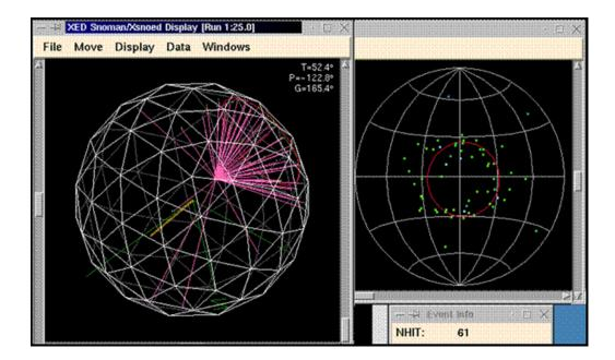
Figure 3: A physics event in SNO's event display. The image on the left shows SNO's PMT support structure and the reconstructed Čerenkov photon trajectories in the event. The image on the right shows the same event projected onto a flat circular surface; the dots indicate hit PMTs. The event vertex and electron direction are reconstructed using the hit PMT locations and times. The electron energy can be estimated by the number of PMT hits.
