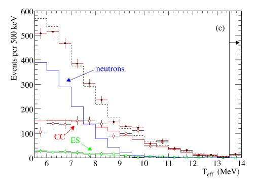
Figure 11: Distributions of electron kinetic energy,  $T_{eff}$ , for neutrons, CC events, and ES events, summed MC PDFs (dashed histogram), and real neutrino data (data points). Events with 14 MeV <  $T_{eff}$  < 20 MeV are combined in the same bin.
