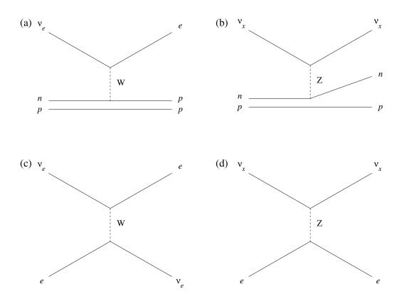
Figure 2: Tree-level Feynman diagrams of the neutrino reactions in SNO. Diagram (a) shows the charged current reaction. Diagram (b) shows the neutral current reaction (resulting in a free neutron). Diagrams (c) and (d) show the graphs that contribute to elastic scattering. Note that only electron neutrinos can scatter from electrons by exchanging a W boson.
