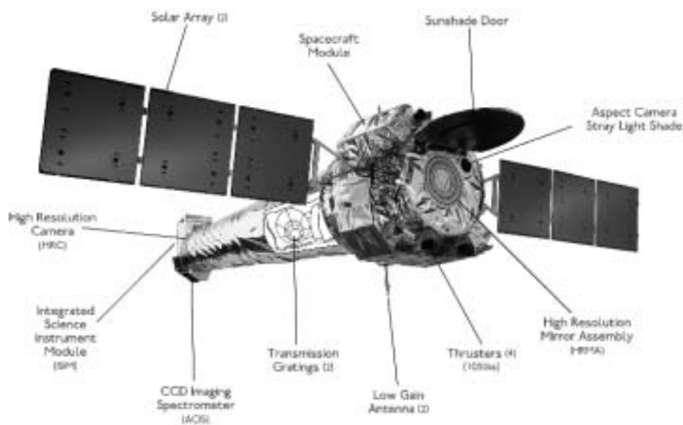
Figure 5: Artist's drawing of the Chandra X-Ray Observatory with major components labeled.
