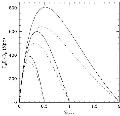
Fig. 2. Shear as a function of lens redshift, for several values of source redshift (which correspond to the right-hand end of each curve). The two curves for each source redshift demonstrate the effect of changing the cosmology, which is nearly degenerate with changing the lens mass. The lensing efficiency is a very broad function, making weak lensing surveys sensitive to a broad range of redshifts.
