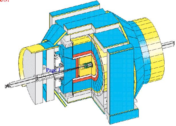
Major systems map to the reconstruction groups Tracking, Calorimetry, and Muon, there are smaller groups for Time of Flight and Luminosity counters
