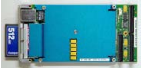
Figure 5: PC architecture Processor PMC board Radisys EPC-6315
