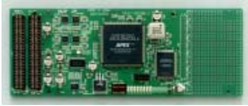
Figure 6: FINESSE-jig, a front-end daughter card for testing system
