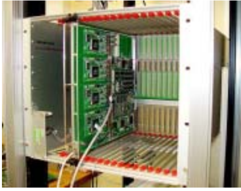
Figure 1: KEK-VME crate with a read-out module
