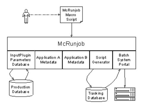
Figure 2: At the direction of the user through a macro script file, one class of Configurators ("InputPlugins") have backends that communicate to external databases, planners, or servers. More conventional Configurators just hold on the application metadata. ScriptGenerators collect results from previous Configurators and produce composite workflows as described above. Finally, a Batch Portal Configurator may take the produced composite script object and submit it to a batch queue.
