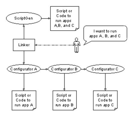
Figure 1: A simple McRunjob scenario. The User or Production coordinator needs to run three applications A, B, and C. The user communicates with the Linker to attach the appropriate configurators, set their metadata values, and run the Linker framework to cause the Configurators to produce jobs.
