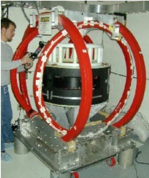
Fig.1 FaroArm Fiducialization of Hall A polarized target.
