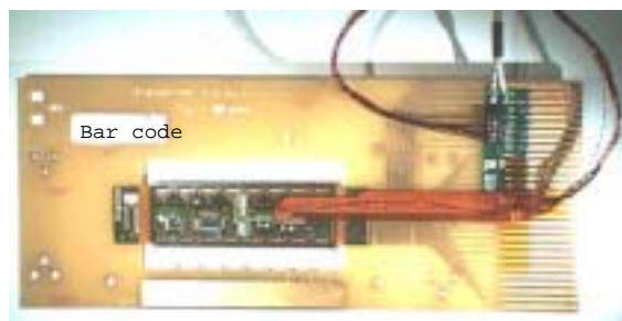
Figure 10: A fully assembled module with disk pigtail and service cable in its PCB frame
