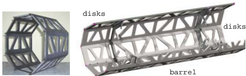
Figure 12: Photo of a life size prototype frame disk section next to computer solid model of entire frame.
