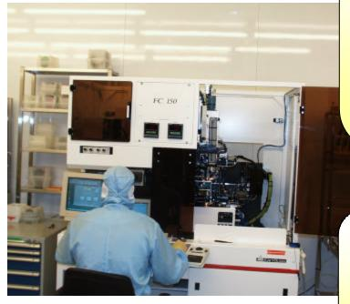
Suss MicroTec FC150 Flip Chip Bonder with both Universal and Solder Reflow Bonding Arms.
