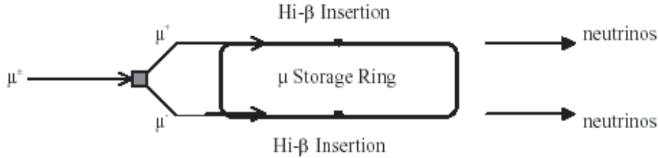
Figure 8: Injection and Circulation of the \mu^\pm in the 32-GeV Storage Ring.
