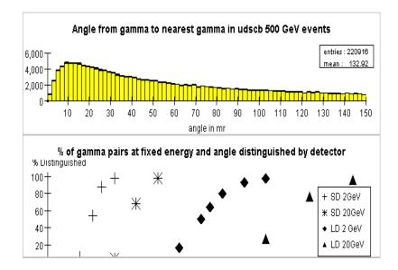
The upper plot illustrates the environment in 500 GeV ee->qq (q=u, d, s, c or b) events with a boost less than 0.2c to eliminate forward events due to ISR down to the Z pole. For each final
