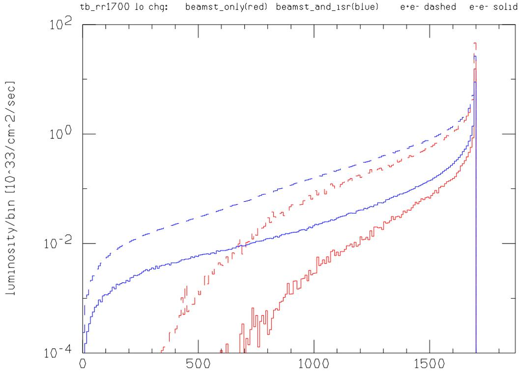
Figure 1: Luminosity spectrum for  $e^+e^-$  (dashed curves) and  $e^-e^-$  (solid curves), for the low-charge design at 1.7 TeV. For each of these cases, we show the spectrum with beamstrahlung only (red), and with both beamstrahlung and initial state radiation (blue).
