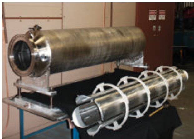
Fig. 8. Stripline kicker system used on ETA-II. A system very similar to this will be deployed on the second axis of DARHT to produce a sequence of radiographic pulses from a 2 μsec pulse in the accelerator.
