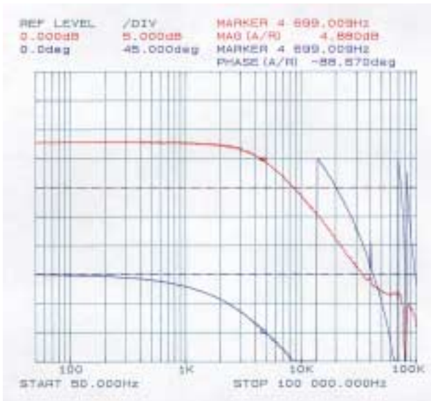
Figure 4: Measured frequency response of FCM with just digital (integrator) control.
