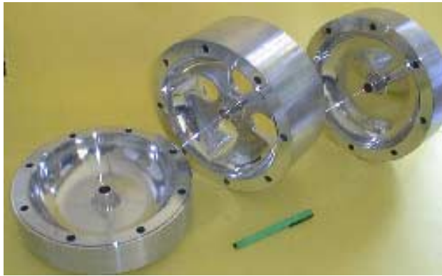
Fig. 6. Trispal cavity cold model. The central piece (with holes) can be removed for 1-cell measurements.
