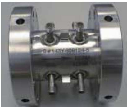
Figure 5. All of the BPMs have a sensitivity of 2.170 \pm 0.005 dB/mm and offsets < \pm 0.5 dB.
