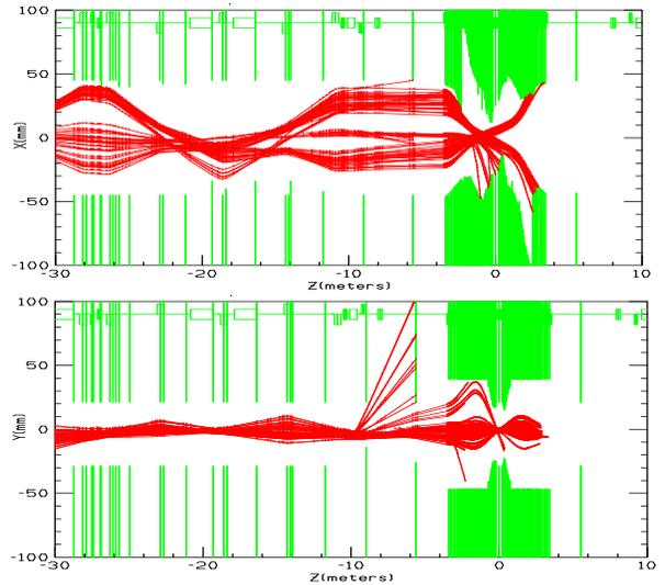
Figure 2: X-Z and Y-Z TOPDRAW plots of Bremsstrahlung particles near the LER IP, located at  $Z = 0$ . Apertures are green, particle tracks are red
