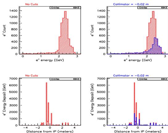
Figure 4: PAW histograms showing decrease in particle count and energy deposited (blue hatching) with collimator cut
