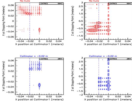
Figure 3: PAW plots of LER beam collimator studies for PEPN, with cuts of particles for  $X \leq 20$  cm
