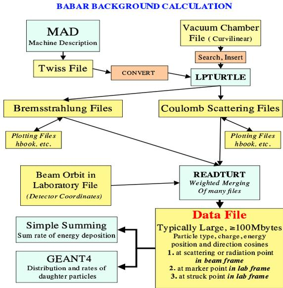
Figure 1: Flow chart of the processes from PEP-II design description to input for GEANT4 background simulations
