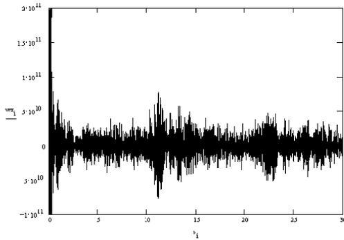
Figure 5: Left: The wake potential, calculated for 30m after the bunch head, plotted against distance from the head of the bunch, abscissa: 0 to 30m.
