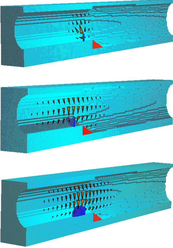
Figure 4: Three versions of the absorber at  $z=-1.75m$ . Top: the original "finger" design - resonant loss=94.5 Watt, frequency=2.58 GHz. Middle: "sector" design - resonant loss=17 Watt, frequency=2.83 GHz. Bottom: "sector with taper" - resonant loss=3 Watt, frequency=2.82 GHz.
