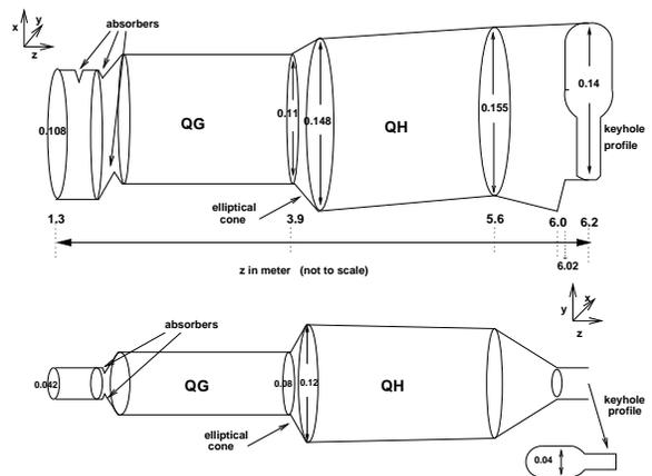
Figure 3: Version II, Superconducting Magnets: A diagram (not to scale) of the beam tube at the Superconducting Magnets . (The last 2 absorbers at the end of the interaction region can be seen at the beginning of this section.)
