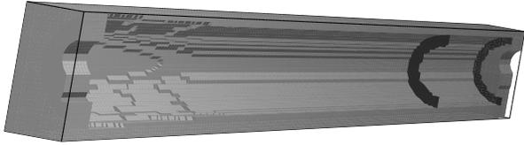
Figure 1: Version I: A foreshortened view of the interaction region at Zeus, the absorbers are shown as dark arcs.
