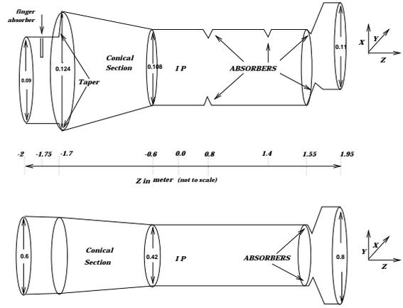
Figure 2: Version II: A diagram of the Interaction Region.
