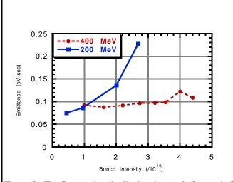
Figure 3. The Booster longitudinal emittance before and after the Linac upgrade.
