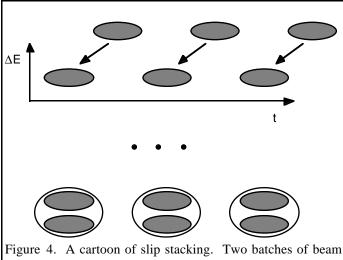
are displaced in azimuth and energy (above), are brought close to each other, and are then combined in a single, large bucket.
