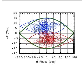
Figure 5. A simulation of slip stacking. The points represent the final phase space coordinates of the particles tracked in the presence of the two rf systems. The smaller curves are the moving rf buckets that would be generated by one system if the other system were not present. The large curve represents the stationary bucket into which most of the particles will be captured.
