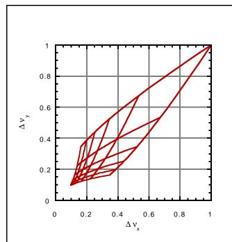
Figure 1. Beam-beam horizontal versus vertical tune. The tune is normalized to a maximum of 1 by the linear beam-beam tune shift (Eqn. 2). The tunes are shown parametrically as a grid lines of constant x or y amplitudes. Amplitudes in the range of 0 to  $5\sigma$  are shown, assuming a beam with a gaussian distribution.
