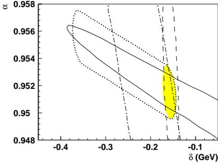
Figure 8: Constraints on slope  $\alpha$  and intercept  $\delta$  from observed  $J/\psi \rightarrow e^+e^-$  (dashed-dotted line),  $\pi^0 \rightarrow \gamma\gamma$  (dashed line), and  $Z \rightarrow e^+e^-$  decays (solid line). The shaded inner contour shows the combined result. The dotted line indicates the allowed area when nonlinear terms, as constrained by test beam measurements, are included.
