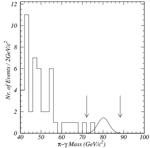
Figure 14: The CDF distribution in  $M(\pi\gamma)$  for the search for the rare decay  $W \rightarrow \pi\gamma$ . The arrows indicate the search window. The Gaussian, centered at  $M_W$ , corresponds to the 95% CL limit of 4.9 events.
