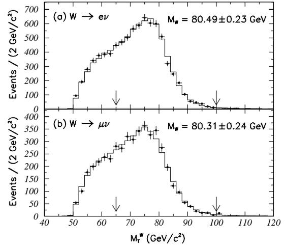
Figure 11: Transverse mass distribution of  $W \rightarrow e\nu$  (top) and  $W \rightarrow \mu\nu$  (bottom) decays from CDF. The points are the data and the histogram is the best fit to the data. The arrows indicate the range used to extract the  $W$ -mass.
