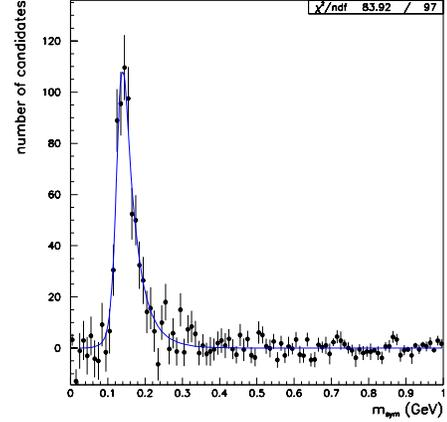
Figure 7: The  $M_{sym}$  mass spectrum obtained from  $\pi^0 \rightarrow \gamma\gamma$  decays.
