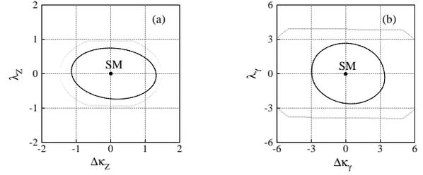
Figure 16: Contour limits on anomalous coupling parameters at the 95% CL (inner curves) and unitarity contours (outer curves) for DØ assuming  $\Lambda = 1.5$  TeV for the process  $WW/WZ \rightarrow e\nu jj$ . SM couplings have been assumed for (a)  $WW\gamma$  and (b)  $WWZ$  vertex.
