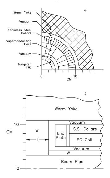
Figure 2: A quarter-section view (a) and an elevation view (b) of a quadrupole magnet for the IR region of the muon collider.
