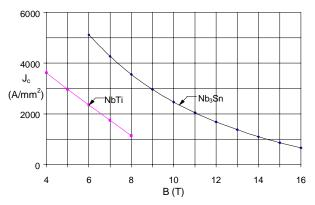
Figure 3: Critical current vs. field for Nb<sub>3</sub>Sn and NbTi superconductors at 4.2 K.
