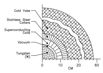
Figure 1: A quarter-section view of a dipole magnet for the muon collider ring.
