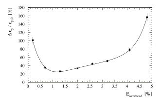
Figure 3: Average emittance growth  $\Delta \epsilon_y/\epsilon_{y,0}$  after beam-based alignment for different BNS configurations. We used an initial quadrupole alignment of 50  $\mu$ m rms, a static BPM to quadrupole offset of 2  $\mu$ m rms, a BPM-resolution of 1  $\mu$ m rms and perfect structure BPM's. The alignment was done in 14 sections and 5 iterations.
