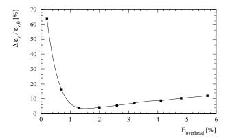
Figure 2: Average vertical emittance growth  $\Delta \epsilon_y/\epsilon_{y,0}$  for the different BNS configurations from Figure 1 and a  $1\sigma$  (2.2  $\mu$ m) initial beam offset. The initial uncorrelated beam energy spread was set to zero.
