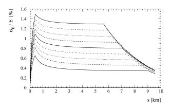
Figure 1: Beam rms energy spread along the linac for different BNS configurations. The energy spread was set to zero at the start and was fixed to about 0.3% at the end, as required by the final focus system. The different BNS configurations are defined in Table III and are referred to as number 1 to 9, where 1 is the lowest curve.
