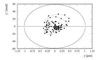
Figure 4: Phase space locations y and y' of the bunches at the end of the linac for a  $1\sigma$  initial vertical beam offset. y and y' are referenced to their average values. The bunch positions are compared to the beam ellipse from the average single-bunch emittance.
