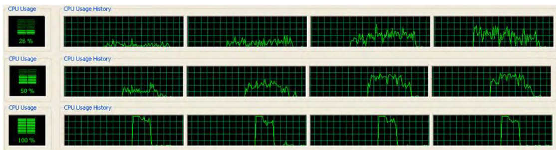
Figure 5: Processor Activity Recordings: These figures show the recorded processor activity on a quad-core processor in a simulated distributed-memory computing environment for one, two, and four processors, respectively. As the number of threads increases, we can note clear increases in processing activity and decreases in computing time.
