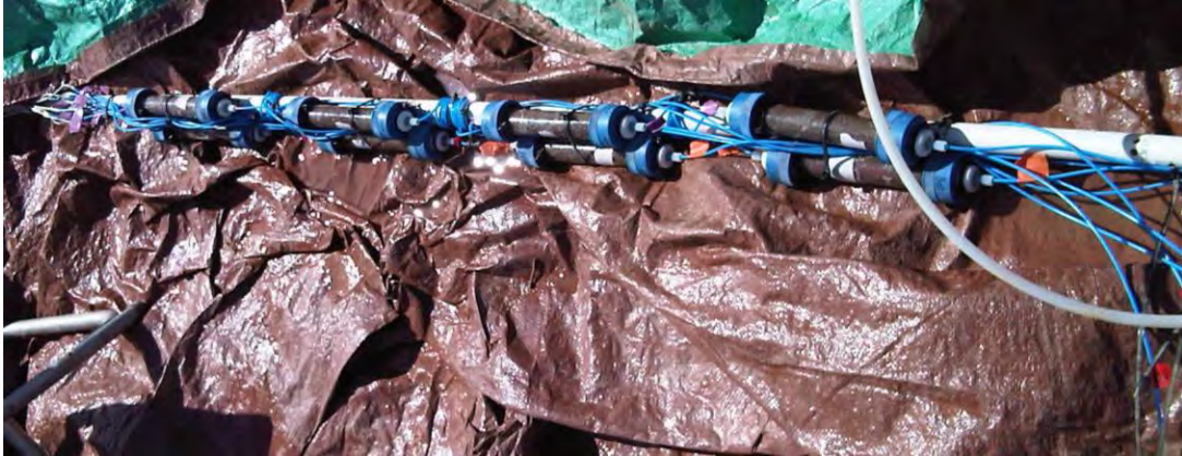
Figure 3: The in-well column setup. The columns are the blue-capped cylinders and are shown filled with sediment. The blue tubing is polyethylene tubing.
