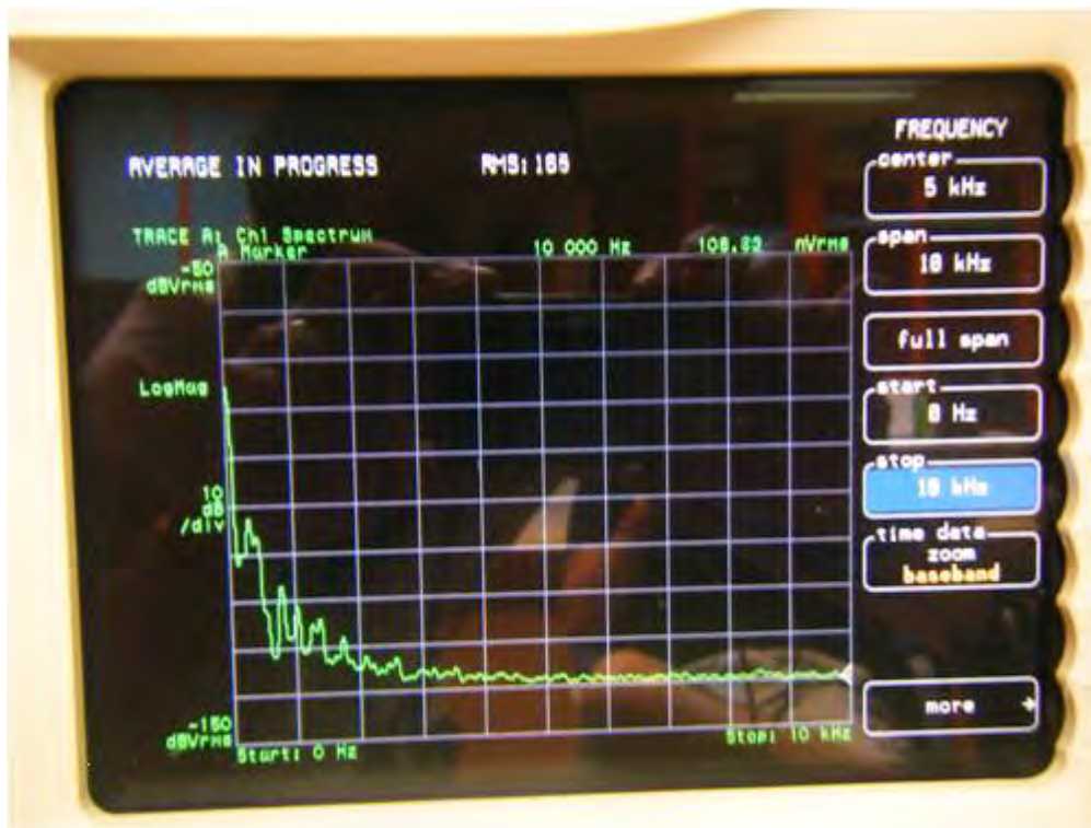
Figure 5. The spectrum analyzer displays a noise plot that resembles a 1/f plot.
