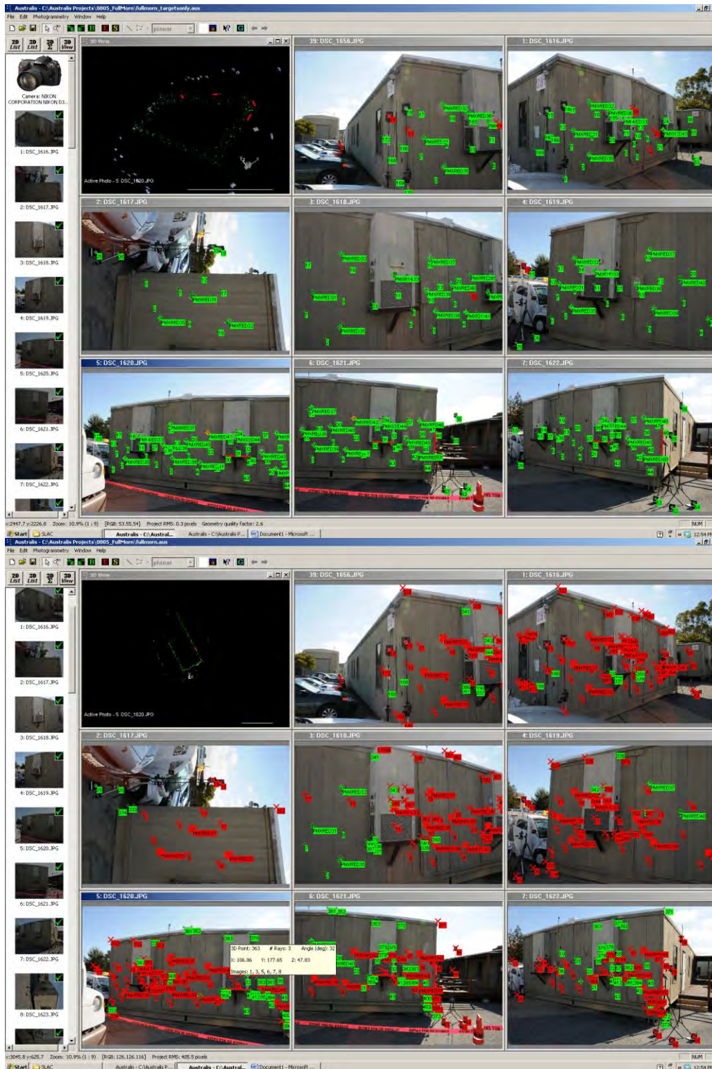
Figure 6 Although Australis has accurately established the a target network for all four exterior walls in the upper screenshot, as more feature points are marked, Australis is no longer able to calculate the position of many of the originally established points. The digital model is deconstructed and the work is irretrievable.
