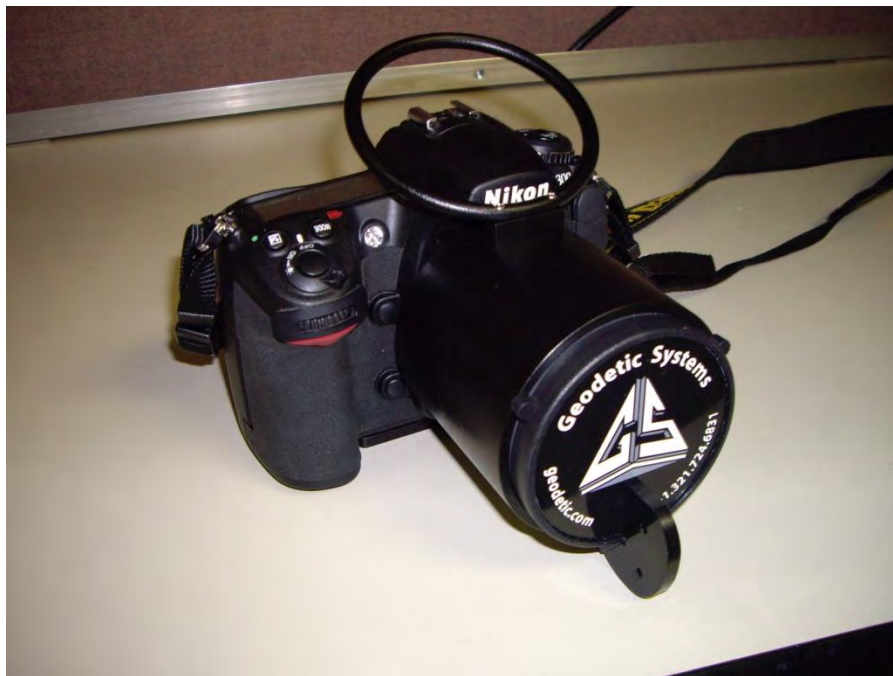
Figure 1 Modified Nikon D300. Several external and internal modifications were made to hold moving parts in place to create a metric camera.
