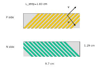
Figure 8: Schematic view of the two sides of the striplets detector.
