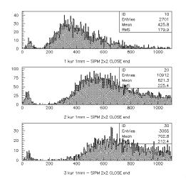
Figure 32: Light collected by 1, 2 and 3 fibers coupled to a SiPM  $2 \times 2 \text{ mm}^2$ .
