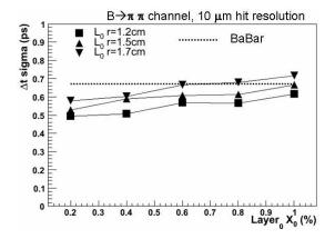
Figure 6: Resolution on the proper time difference of the two B mesons ( $\beta \gamma = 0.28$ ), for different Layer0 radii, as a function of Layer0 thickness (in  $X_0$  %).
