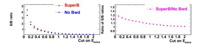
Figure 28: Left: Signal-to-background ratio with and without a backward calorimeter, as a function of the  $E_{\text{extra}}$  selection. Right: Ratio of the S/B ratio with a backward calorimeter to the S/B ratio without a backward calorimeter, as a function of the  $E_{\text{extra}}$  selection.
