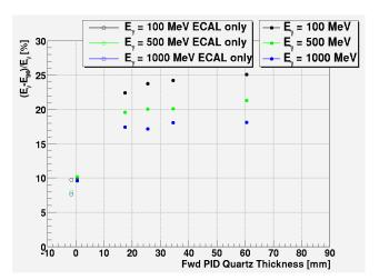
Figure 25: The effect of quartz material in front of the forward calorimeter, as a function of thickness and photon energy. The ordinate is  $f_{90}$ , explained in the text, expressed as per cent.
