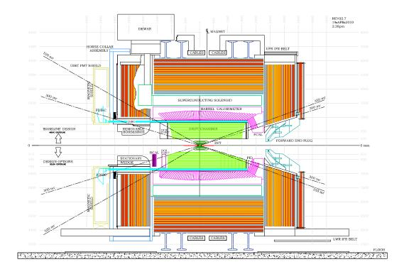
Figure 1: Concept for the SuperB detector. The upper half shows the baseline concept, and the bottom half adds a number of optional detector configurations.
