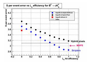
Figure 7:  $\sin 2\beta_{eff}$  per event error as a function of the Layer0 efficiency for the different options (i.e. different material budget).
