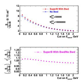
Figure 3: Top:  $S/\sqrt{S+B}$  as a function of the cut on  $E_{extra}$  with (circles) and without (squares) the backward EMC. Bottom: ratio of  $S/\sqrt{S+B}$  for detector configurations with or without a backward EMC as a function of the  $E_{extra}$  cut.
