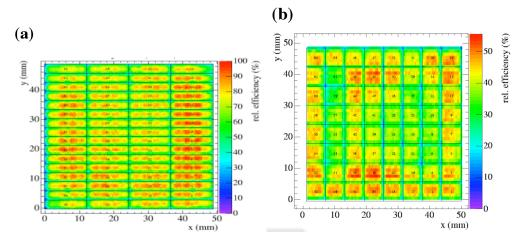
(a) Single photoelectron response of H-9500 (b) Similar scan of H-8500 MaPMT with pix-MaPMT with  $3 \,\mathrm{mm} \times 12 \,\mathrm{mm}$  pixels. els:  $6 \,\mathrm{mm} \times 6 \,\mathrm{mm}$ .
