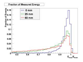
Figure 24: Ratio of the measured/beam energy in the forward calorimeter for 100 MeV photons and two different thickness of quartz, as well as no quartz, in front of the calorimeter.
