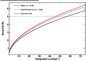
Figure 2:  $S/\sqrt{S+B}$  of  $B \to K\nu\bar{\nu}$  as a function of the integrated luminosity in three different detector configurations.
