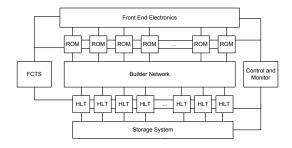
Figure 40: High-level logical view of the Online System
