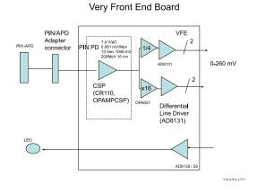
Figure 21: Block diagram for the Very Front End board, for the barrel and forward endcap signal readout.
