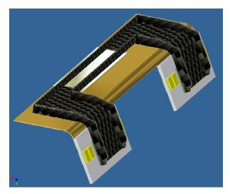
Figure 9: Mechanical structure of a striplets Layer0 module.
