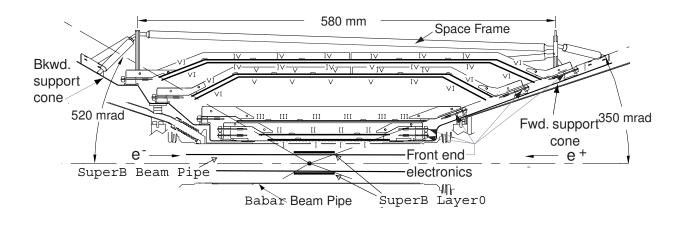
Figure 5: Longitudinal section of the SVT
