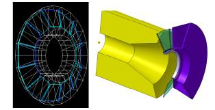
Figure 20: Left: the "DIRC-like" TOF design, as currently implemented in Geant4 simulations. Right: a possible design for the mechanical integration of this detector (in green) in SuperB. The yellow (magenta) volumes represent the envelope of the DCH (forward EMC).
