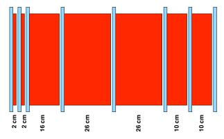
Figure 30: Sketch of the longitudinal segmentation of the iron absorber (red) in the baseline configuration. Active detector positions are shown in light blue from the innermost (left) to the outermost (right) layers.
