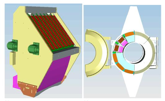
(a) Mechanical enclosure and support of the (b) Overall mechanical support design with the FBLOCK with the new wedge. new magnetic shield door.
