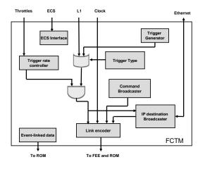
Figure 36: Fast Control and Timing Module
