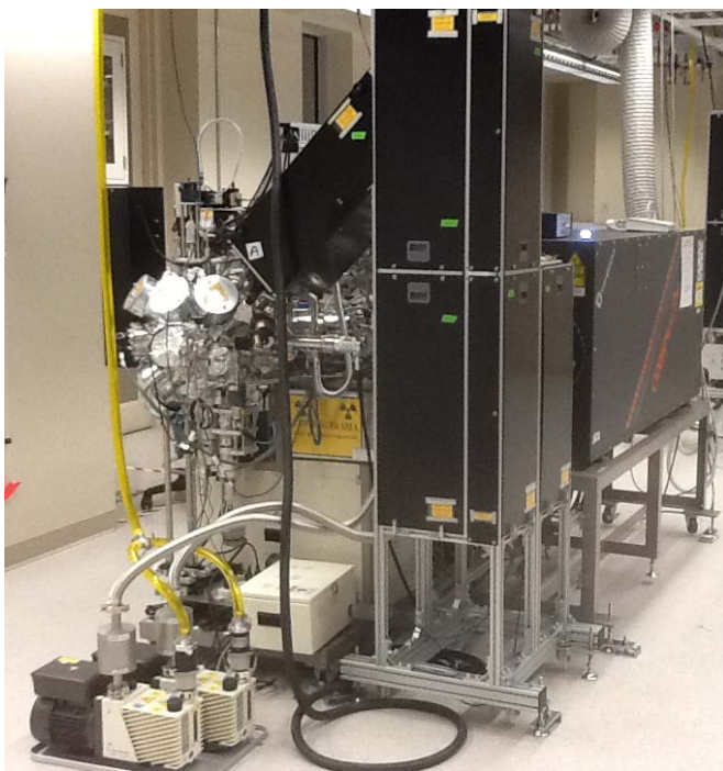
Fig. 1: Completed pulsed laser deposition system and integrated laser.
