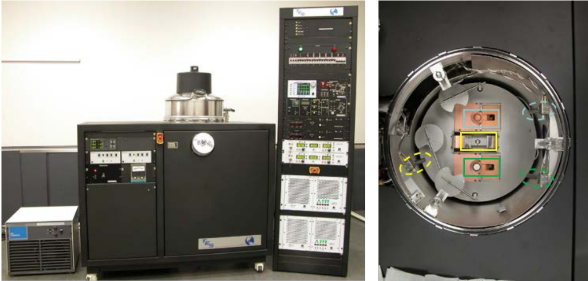
Figure 1: Fully assembled three source PVD system (left). Each source (solid rectangle) has its own corresponding QCM (dashed oval) for deposition rate control.
