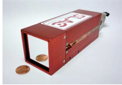
Fig. 1: a) ePix 10k sensor: designed and fabricated in house at SLAC and SNF. b) ePix-ONE camera assembly.
