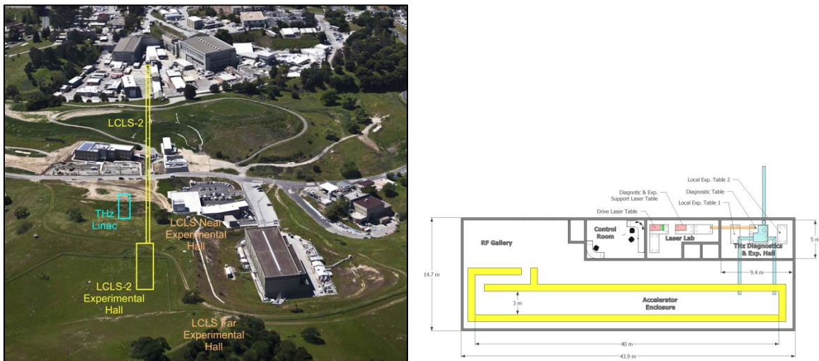
Figure 5: Layout of the proposed THz facility. The facility would be located adjacent to LCLS I and II. The accelerator enclosure could be much more compact for the X-band accelerator option.
