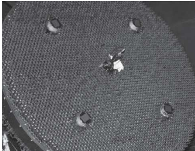
Figure 5.18: Photograph of the LAMOST focal plane with star guiders.
