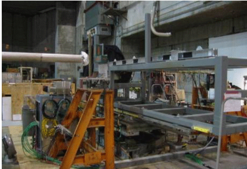
Figure 16.10: Picture of the actual beam test setup in Endstation A. The aluminum pipe is the end of the beam line delivering 10 GeV electrons. The Focusing-DIRC prototype is mounted on the steel structure, the PCB is covered with a black cloth.
