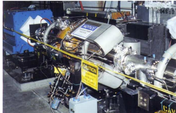
Figure 3.8: Installed PEP-II cavity with damping waveguides.
