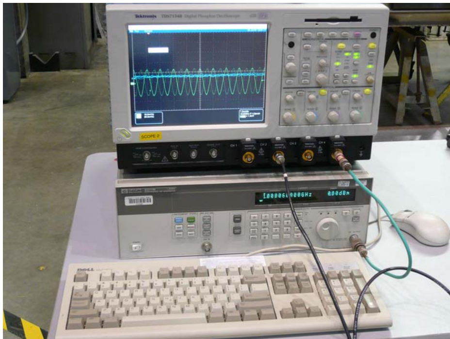
Figure 1: The general setup for the biconical calibration. (a) Left: The yagi. Right: The biconical. (b) The oscilloscope on top of the signal generator.
