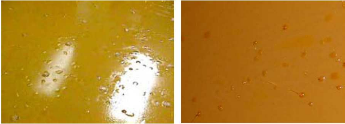
Figure 2.20: Surface image of a bad RPC
