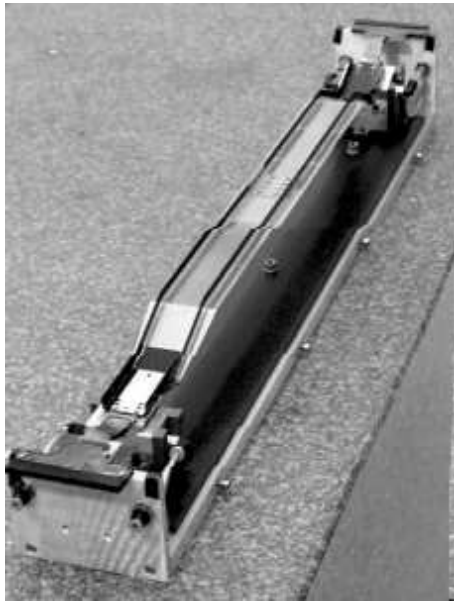
Figure 2.7: Photograph of an SVT arch module in an assembly jig.
