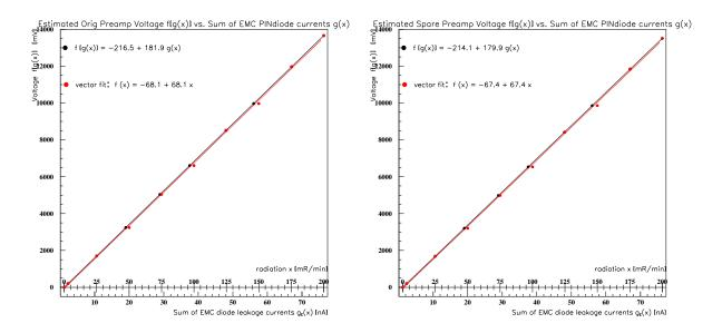
Figure A.15: Final estimate of preamplification boards output w.r.t input currents from the EMC PIN-diode sensors, and w.r.t radiation, for the original preamplification board (left) and the spare preamplification board(right).
