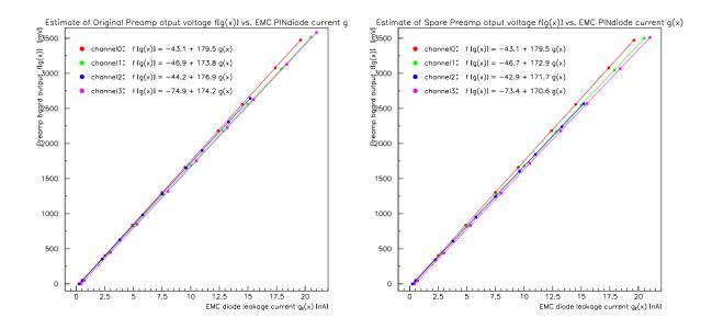
Figure A.12: Estimate of preamplification board output voltage vs. currents for single EMC PIN diodes (original preamplification board to the left, spare preamplification board to the right).
