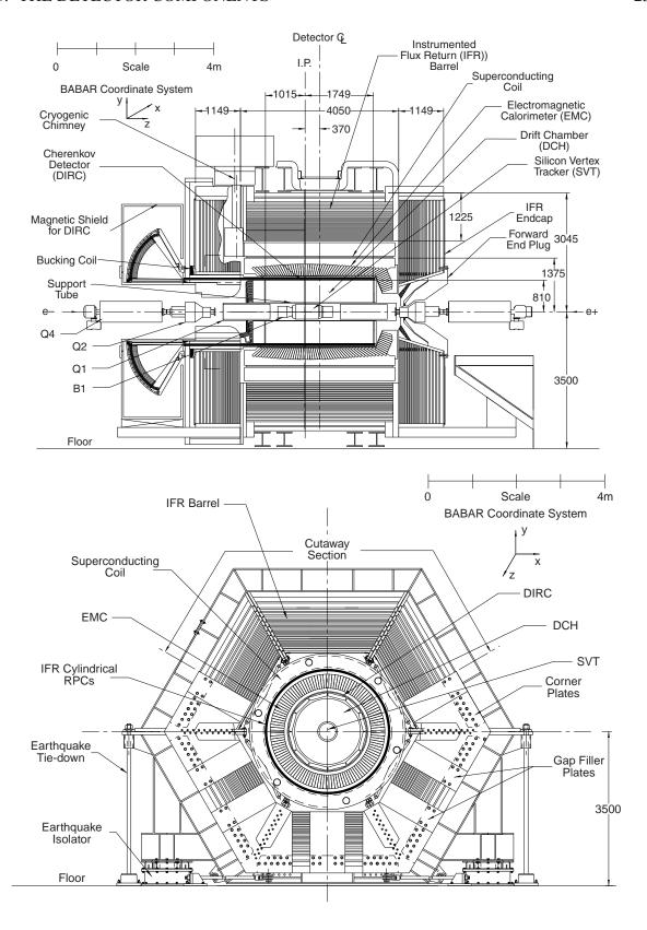
Figure 2.3: BABAR detector, side view (top) and end view (bottom).
