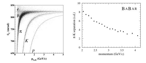
Figure 2.6: The DIRC provides  $K/\pi$  separation from about 500 MeV/c up to the kinematic limit of about 4.5 GeV/c.
