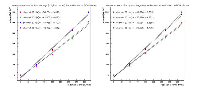
Figure A.14: Original Pre-Amplifier Board output vs. radiation (measured), to be compared with the  $f_o(x)$  entries for channels 0 - 3 for the old DCH sensors in table A.5.
