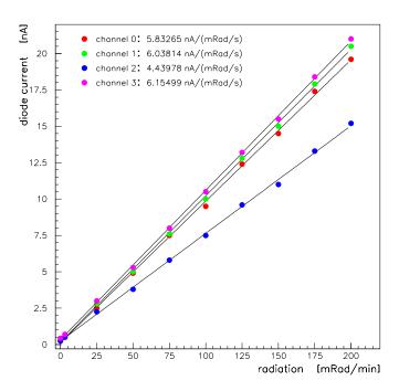
Figure A.8: Measured leakage current vs. radiation for the new EMC PIN-diode sensors biased at 30 V.
