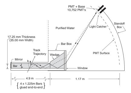
Figure 2.5: Schematic concept of the DIRC. Cherenkov light released in the silica material is guided towards the back of the detector where 10752 photo-multiplier tubes record the signals and and allow for reconstruction of the characteristic Cherenkov ring images used in particle identification.
