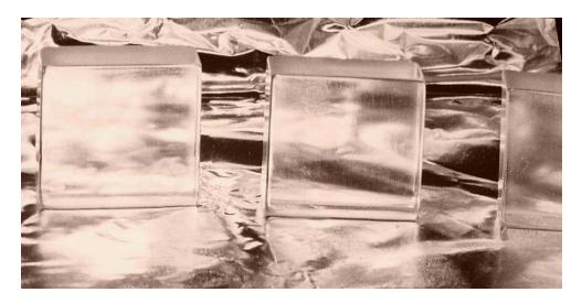
Figure A.2: New CsI(Tl) crystals in the process of being polished. The crystals are  $4 \times 4 \times 1$  cm<sup>3</sup> blocks of scintillating material providing high photon yield for PIN-diode readout.
