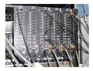
Figure A.6: CAMAC Beam Abort Module in the IR-2 alcove.
