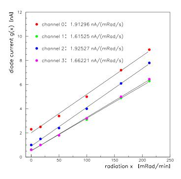
Figure A.9: Measured leakage current vs. radiation for each of the old DCH PIN-diode sensors biased at 30 V.
