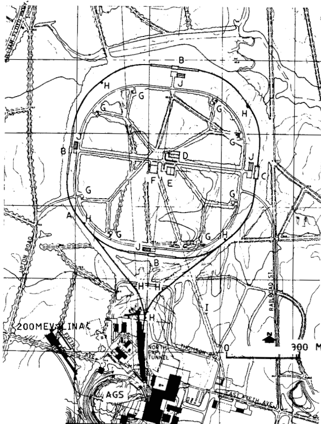
Fig. 1. ISA Site Plan. Legend: A-main magnet enclosure, B-large experimental halls, C-small experimental hall, D-compressor building, E-service building, F-69 kV substation, G-refrigerator buildings, H-exit buildings, I-69 kV overhead line, J-assembly buildings.
