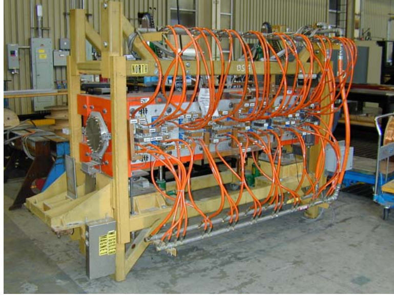
Figure 4.11: Photograph of our magnet rewired as a chicane. The orange hoses are for water cooling. On the front face is one of the two added flux return plates.
