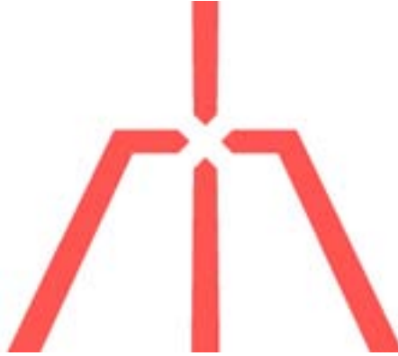
Figure 3.8: Zoom in of Hall probe shallow etch pattern for a 0.5\ \mu\text{m} Hall probe.
