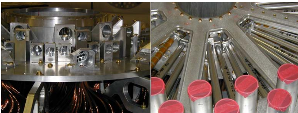
Figure 3.22: ( left ) Mirrors; ( right ) air light guides; The phototube assemblies are inserted inside the cylinders shown here.
