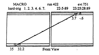
FIGURE 6. MACRO's first upward going muon event. The circles indicate the scintillation counters struck by the muon and the dots correspond to the streamer tube "hits" along its trajectory. The numbers shown are the relative times in nsec with an arbitrary offset of the pulses detected in the given scintillation counter. This particle has an upward velocity of  $\beta = 0.995$ .
