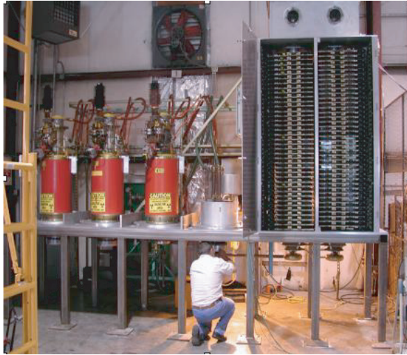
FIGURE 3.42. Photograph of the NLC induction modulator with three of the SLAC 5045 klystrons that are used as a load.
