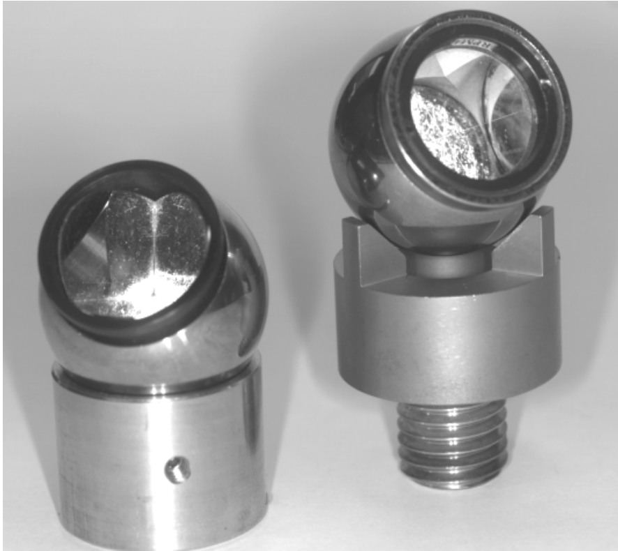
Figure 12.4 Sphere mounted glass and air reflectors
