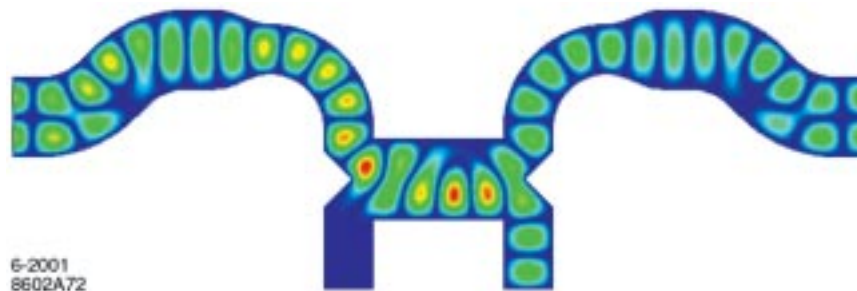
Figure 4.23: A 3-dB tap-off made with a ‘magic H’ hybrid and jog converters. Electric field patterns are shown for power flow from left to right.
