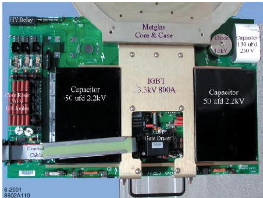
Figure 4.7: Induction cell driver board.
