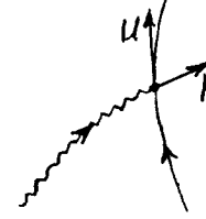
Fig. 4. The interaction of a photon of four-momentum \mathbf{p} with a detector of four-velocity \mathbf{U} .
