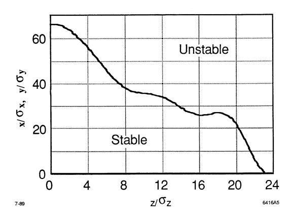
Fig. 5. The dynamic aperture of the ring with the noninterlaced sextupoles. This is examined by a particle-tracking of 1,000 turns with the synchrotron motion.
