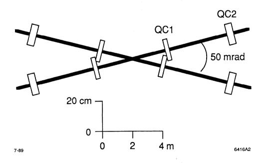
Fig. 2. Design of the IP region with a horizontal crossing angle. The separate final quadrupoles are used for both beams, and no separation device is required.
