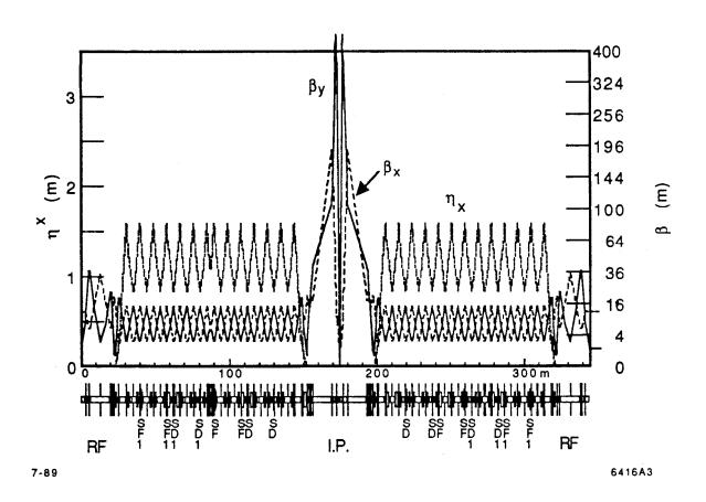
Fig. 3. Optics for the  $\tau$ /charm factory. This ring is placed in a horizontal plane and has a near race-track shape. One of the arc(left) is lengthen to break the symmetry and avoid the extra intersections of the two rings.
