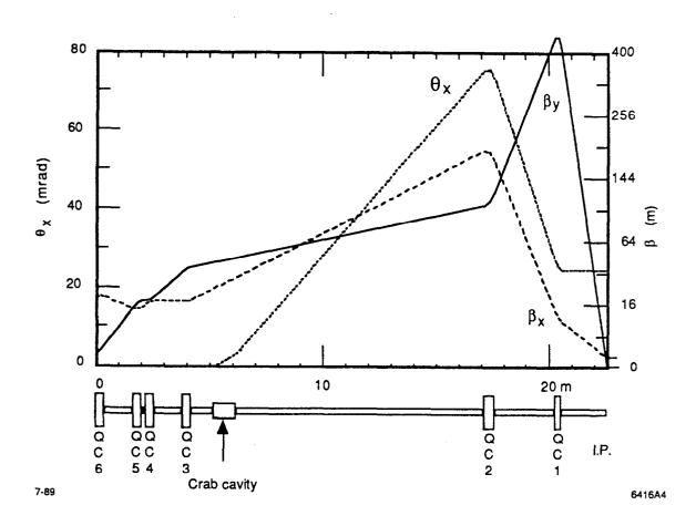
Fig. 4. The crab cavity and the induced crab angle  $\theta_x$  around the IP.
