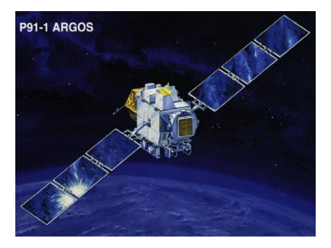
Figure 3.1: An Artist's rendition of ARGOS. The rectangular object on the side of the satellite facing out of the page is the USA experiment.
