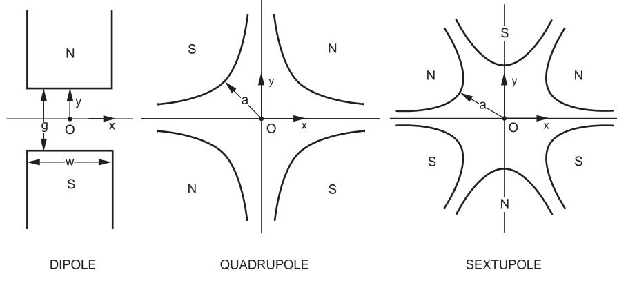
Illustration of the magnetic midplane (x axis) for dipole, quadrupole and sextupole elements. The magnet polarities indicate multipole elements that are positive with respect to each other. The coordinate system is right-handed, so that the beam particles will be emerging from the paper and moving into the face of the reader.
