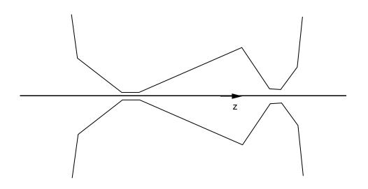
A cross section of a neutrino horn in the z - r plane.
