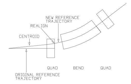
The effect of the **REALIGN** command in the data above can be shown by the following figure:
