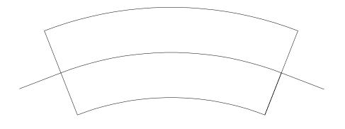
An SBEND Type of Bending Magnet
