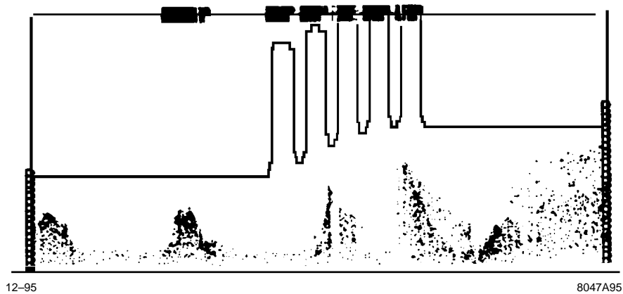
Figure 8-33. Computer simulation of bunched beam passing through the X5011 disk-loaded output circuit. The vertical scale is magnified by 3 to emphasize the growth of bunch amplitude in the output circuit.
