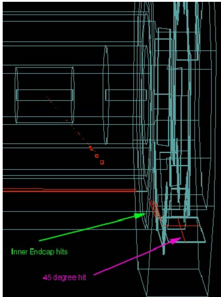
Figure 5.3 – Muon event showing inner endcap and 45DC hits.
